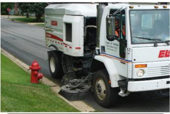
Brian Reynolds operates a regenerative air sweeper on the streets of Vienna. The vehicle blows hurricane force air down on one side and vacuums on the other side to create a turbulent suction which not only collects what the brush dislodges but also fine dust and particles. The technology is environmentally friendly and superior to the previous generation of sweeper which used a conveyor belt to carry the debris into a hopper.
