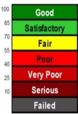
US Army Corps of Engineers Pavement Condition Index (PCI) Scale
