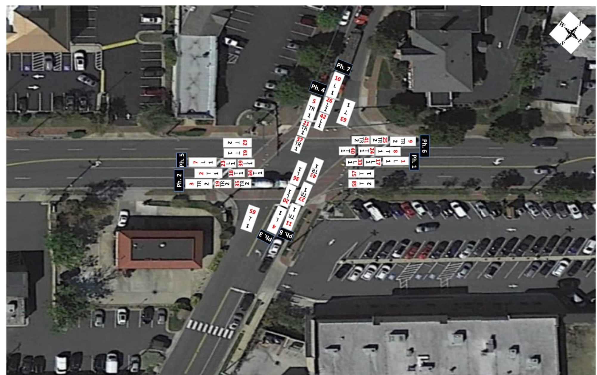
Maple Avenue West (Rte. 123) at Nutley St (Rte. 243) Detector Channel Assignments for ATSPM
