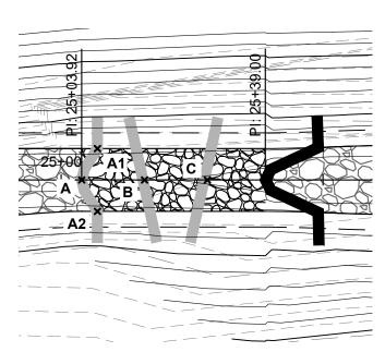
NOTE: FOR CONSTRUCTED RIFFLES, LOGS MAYBE ELIMINATED FROM RIFFLE MATRIX IF THERE IS NOT ENOUGH SPACING FOR CONSTRUCTION. FIELD ENGIENEER AND TOWN OF VIENNA WILL MAKE DETERMINATION IF LOGS ARE ELIMINATED.
