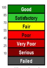
US Army Corps of Engineers Pavement Condition Index (PCI) Scale
